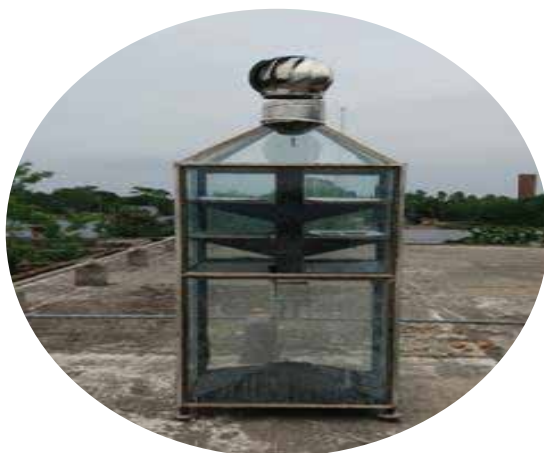
Fig. 1. Wind existed solar cum mechanical dryer. Wind operated exhaustor has been placed at the top of the dryer
