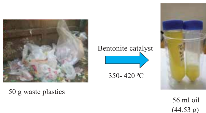
Fig. 4. Converting waste plastics into oil by bentonite catalyst under inert atmosphere
